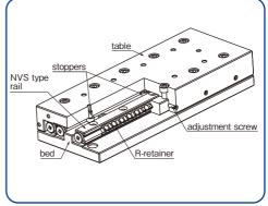
The NVS type utilizes stainless steel rails The NVTS type utilizes NVS type Slide Way and resin retainers, which is suitable for between aluminum table and aluminum bed. anti-corrosion requirements.
