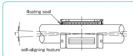
Figure D-3 Basic Structure of TK
