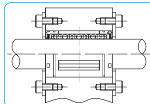
Figure D-5 Clearance Adjustable Type
